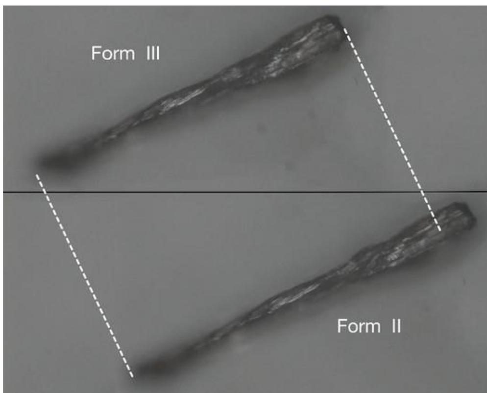
**Figure 1.** Change of the crystal's microscopic dimension during the thermosalient phase transition.
