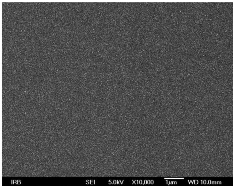
**Figure 2.** AZO thin film, annealed at 400°C, heating rate 2°C per minute.
