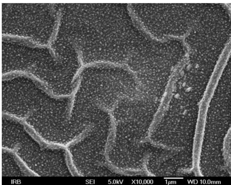
**Figure 1.** AZO thin film, annealed at 500°C, heating rate 50°C per minute.
